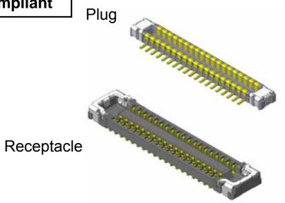
The WP27D Series is a 0.35mm pitch low-profile stacking type board-to-board (FPC) connector with special hold-downs that can be used as power supply terminals, and is ideal for high-density mounting in slim and compact information communication devices like smartphones. This product has a structure that adds protection to the mating surface to prevent damage to the insulator in case force is applied while connectors are misaligned. Also the hold-downs can be used as high-current terminals.
