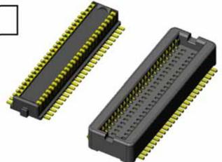
The AC01 series is a 0.5mm pitch horizontal board to board connector, suitable for information and communication equipment, and various other industrial equipment. The connector series are available in 2.5mm and 3.0mm stacking heights, as well as utilizing a highly stable and reliable contact structure which has been proven over decades of use.
