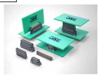
The MA01 Series is the next generation floating board-to-board connector. This product features a highly reliable two-point contact structure, achieving high-speed transmission exceeding 8Gbps. With an operation temperature range of -40 to 125 the connector is suitable for harsh temperature environments unique to the automotive industry.
