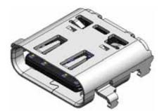
The DX07 Series connectors are USB Type-C® compatible connectors which are used in various consumer and industrial devices which require a power and serial data interface. This product is a USB4 specification compatible 2-row SMT type receptacle connector which can support data rates up to 40Gbps. New features introduced with the USB4 specification such as tunneling of various signals is also supported.
