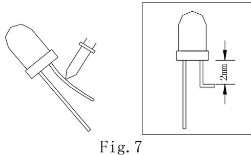
2) Forming lead should be carried out prior to soldering and never during or after soldering.
