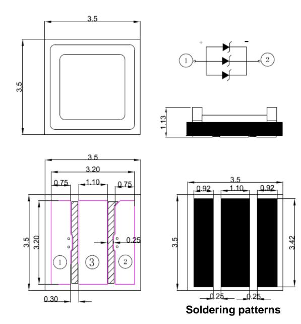
1. Dimensions are in millimeters.
