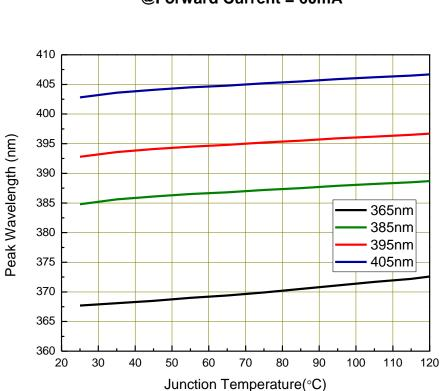
Peak Wavelength vs. Junction Temperature @Forward Current = 60mA
