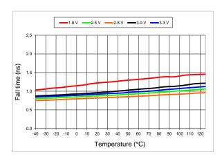
Figure 12. 20%-80% Fall Time vs Temperature
