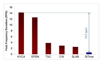
Figure 6. Shock Robustness<sup>[6]</sup>
