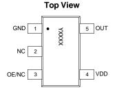
Figure 1. Pin Assignments
