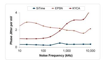
Figure 4. Power Supply Noise Rejection<sup>[4]</sup>
