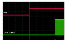
Figure 16. Startup Waveform vs. Vdd
