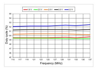
Figure 10. Duty Cycle vs Frequency
