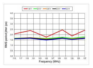
Figure 9. RMS Period Jitter vs Frequency
