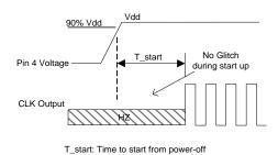
Figure 4. Startup Timing (OE Mode)[7]
