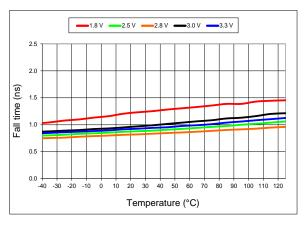
Figure 12. 20%-80% Fall Time vs Temperature
