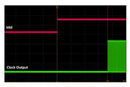
Figure 16. Startup Waveform vs. Vdd
