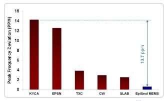
Figure 4. Power Supply Noise Rejection [4]
