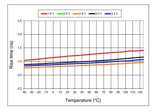
Figure 11. 20%-80% Rise Time vs Temperature
