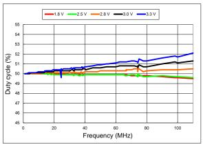
Figure 10. Duty Cycle vs Frequency
