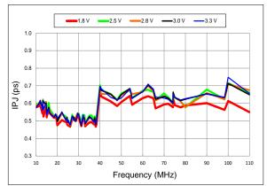
Figure 13. RMS Integrated Phase Jitter Random (12 kHz to 20 MHz) vs Frequency<sup>[9]</sup>
