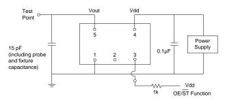
Figure 2. Test Circuit
