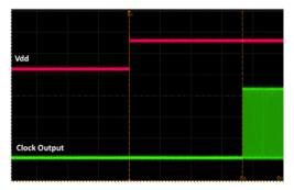
Figure 16. Startup Waveform vs. Vdd
