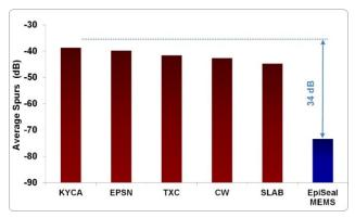
Figure 5. Vibration Robustness<sup>[5]</sup>
