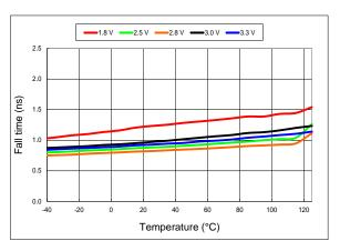
Figure 12. 20%-80% Fall Time vs Temperature
