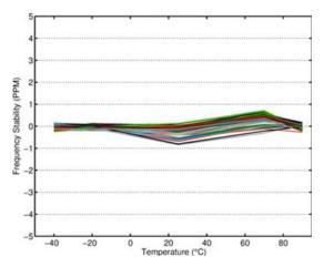
Figure 3. Frequency Stability over Temperature
