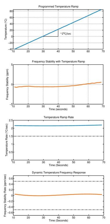
Frequency accuracy under a moderate temperature ramp up to 2°C/sec is limited by the TCXO's trimmed accuracy of the frequency stability over-temperature.
