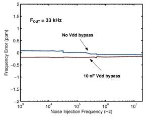
Figure 5. Power Supply Noise Rejection
