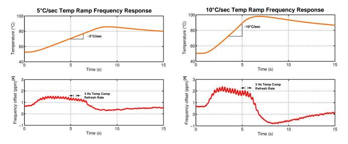
For temperature ramps >5°C/sec, the frequency accuracy is limited by the update rate of the temperature compensation path (see the 5°C/sec and 10°C/sec plots).
