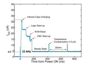
Figure 4. Start-up and Steady-State Current Profile
