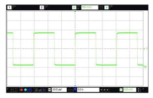
Figure 10. LVCMOS Output Waveform (Vswing = 1.8V, SiT1630AI-H4-DCC-32.768)
