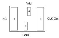
Figure 2. Pin Assignments
