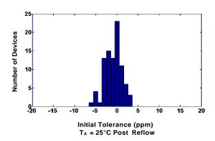
Figure 5. Initial Tolerance Histogram
