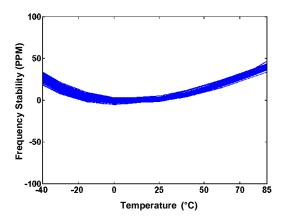
Figure 6. Frequency Stability Over Temperature
