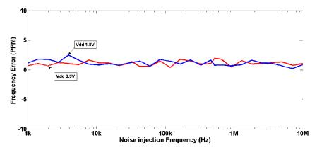
Figure 9. Power Supply Noise Rejection (±150mV Noise)
