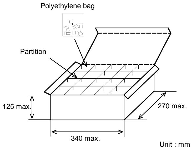
$$\text{The number of packing} = \frac{\text{Packing quantity}}{\text{n}}$$
