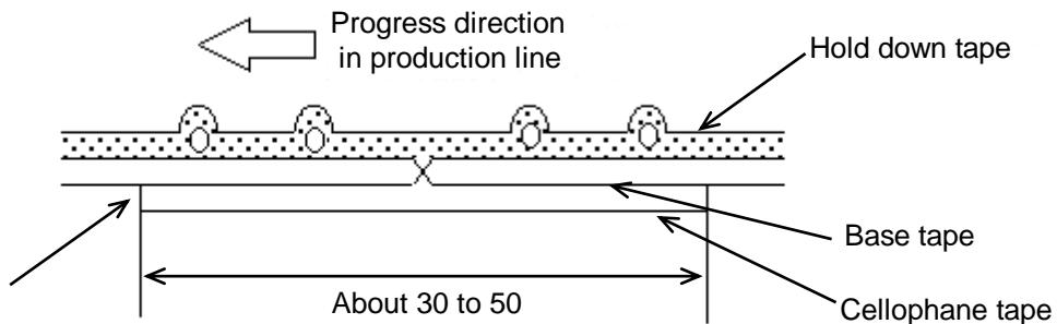
No lifting for the direction of progressing
