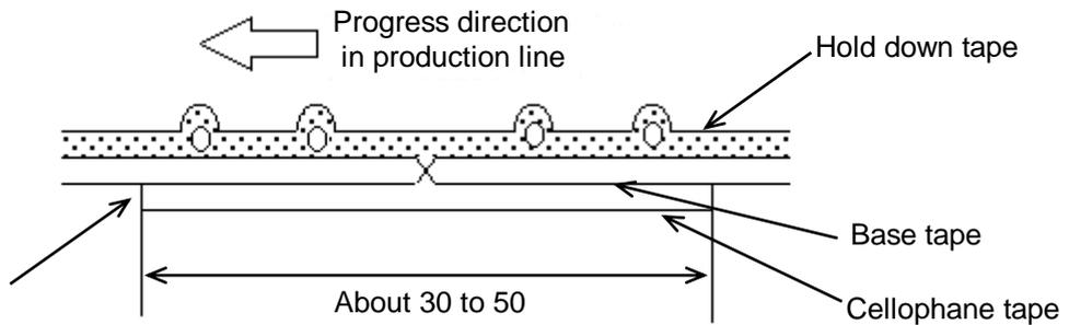
No lifting for the direction of progressing
